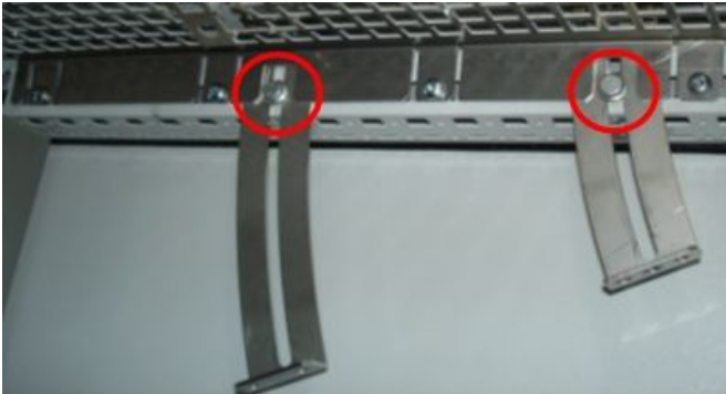
Figure 4: Right bracket bolts, roof folded down
